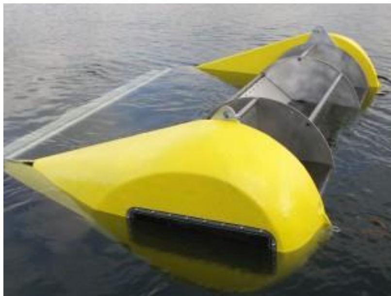
Figure 51: Hydrovolts [29] Class II Turbine 1 - 10 kW capacity depending on flow. Photo courtesy of Hydrovolts Inc. [32]
