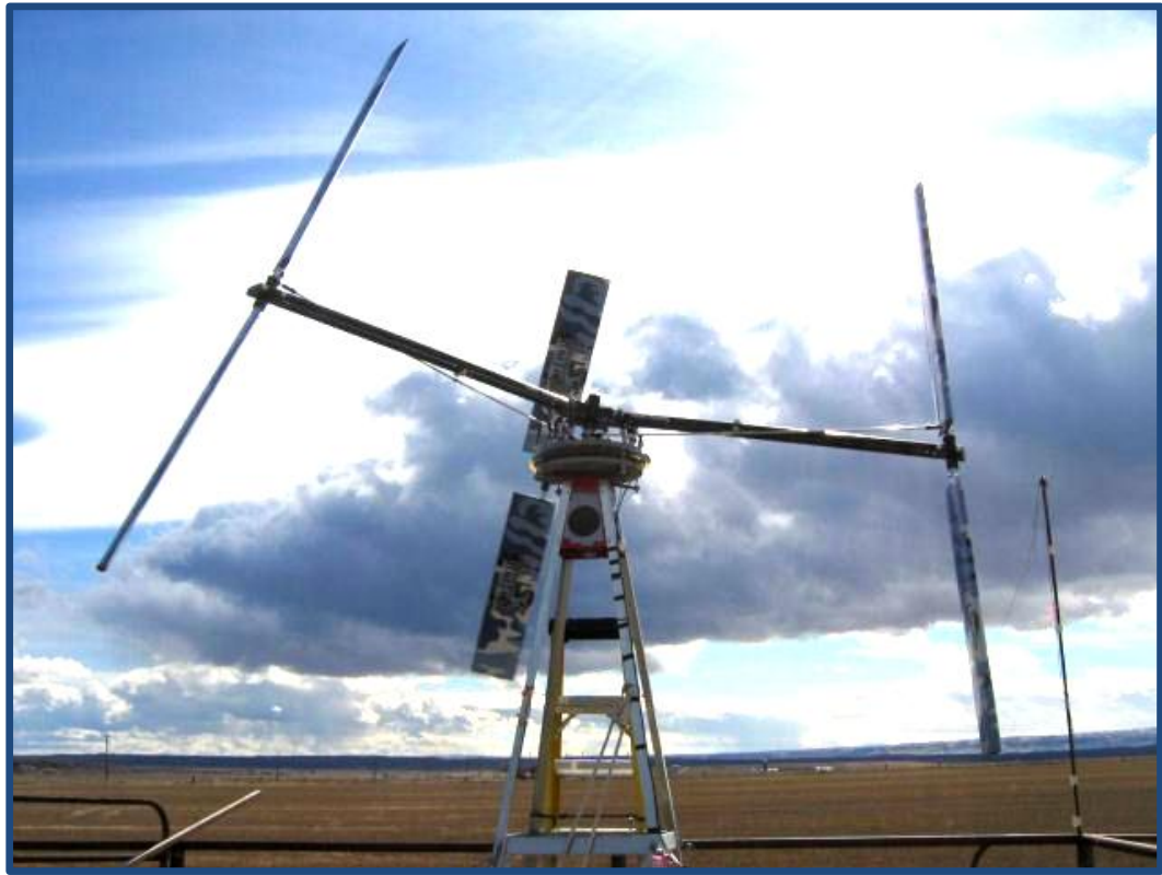
Figure 46: Close-up of a BlackHawk TR-10 VAWT developed by Bruce Boatner [21] showing tilt and articulation
